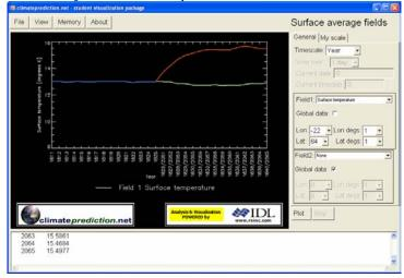
Click on 'global data' for field 1, and then enter the grid reference for your location in the world. 'Lon degs' and 'Lat degs' should stay as 1 degree.
