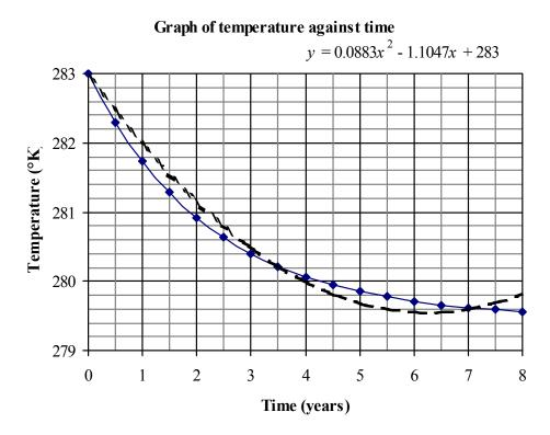
The next graph shows the **cubic** function (dotted line) given by Excel to model the data:
